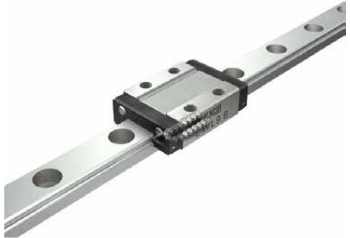
Figure 2. The LWL miniature linear motion rolling guide incorporates two rows of steel balls arranged in four-point contact with the raceways to provide stable accuracy and rigidity.
