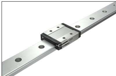
Structured with two rows of balls that make contact with the raceway at four points, linear motion rolling guides are able to deliver high stability and accuracy.
