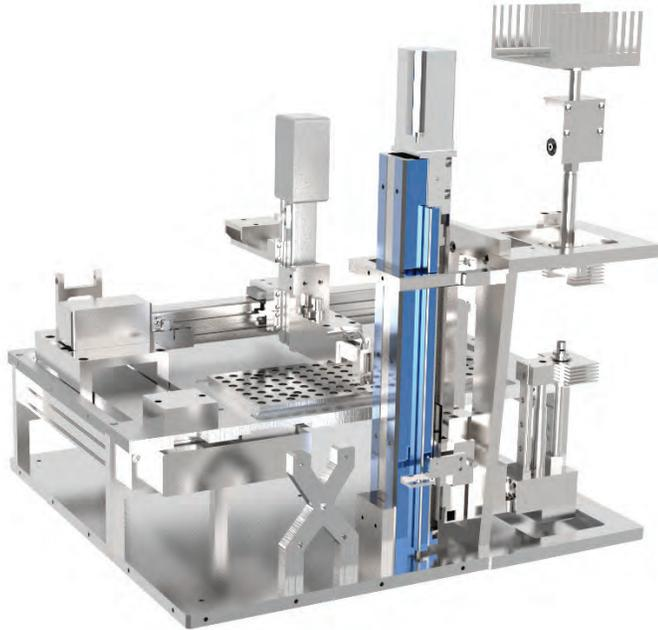
*Wildcat Technologies uses IKO's 10 mm lead positioning tables in their HAWK instrument design.*
