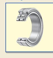
Roller Bearings, in which rollers are incorporated in double rows, are non-separable heavy-duty bearings. They can withstand not only radial loads but axial loads as well, which are supported at the contacts between the shoulders of inner and outer rings and the end faces of rollers. Therefore, they are most suitable for use at the fixing side of a shaft.
