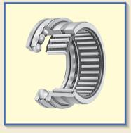
Combined Type Needle Roller Bearings are combinations of a radial bearing and a thrust bearing. Caged Needle Roller Bearings are used as radial bearings and Thrust Ball Bearings or Thrust Roller Bearings are used as thrust bearings. They can be subjected to radial loads and axial loads
