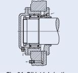
Fig. 24 Oil jet lubrication
