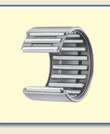
Shell Type Needle Roller Bearings are lightweight with the lowest sectional height among needle roller bearings with outer ring, because they employ a shell type outer ring made from a thin special-steel plate which is accurately drawn, carburized and quenched.
