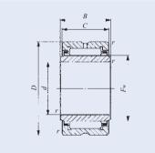
Fig. 7 Machined Type Needle Roller Bearing
