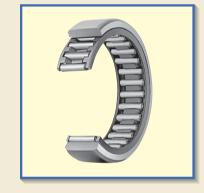
In Needle Roller Bearings with Separable Cage, the inner ring, outer ring and Needle Roller Cage are combined, and they can be separated easily. This type has a simple structure with high accuracy. In addition, the radial clearance can be freely selected by choosing an assembly combination.
