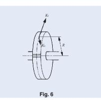
In this case, the resultant normal force on the tooth surface acts as the radial force to the shaft and the magnitude of vibration or shocks varies depending on the accuracy and surface finish of the gear. Therefore, the radial load  $K_r$  applied to the shaft is obtained from the following equation, multiplying the resultant normal force  $K_c$  on gear tooth surface by the gear factor  $f_z$  shown in Table 8.
