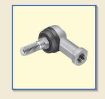
L-Balls are self-aligning rod-ends consisting of a special zinc die-cast alloy body and a studded ball which has its axis at right-angles to the body.
