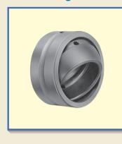
Spherical Bushings are self-aligning spherical plain bushings, which have inner and outer rings with spherical sliding surfaces. They can take a large radial load and a bi-directional axial load at the same time. They are divided into steel-on-steel types that are suitable for applications where there are alternate loads or shock loads, and maintenance-free types which require no lubrication.
