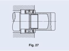
When press fitting, the friction of the fitting surfaces can be reduced by applying high viscosity oil over the fitting surfaces.
