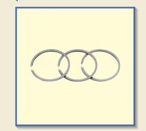
Cir-clips for Needle Roller Bearings have been specially designed for needle roller bearings on which, in many cases, generally available Cir-clips cannot be used. They have a low sectional height and are very rigid. There are Cir-clips for shafts and for bores, and they are used for positioning to prevent bearing movement in the axial direction.
